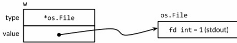
Figure 7.2. An interface value containing an *os.File pointer.
