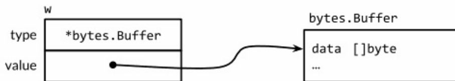
Figure 7.3. An interface value containing a *bytes.Buffer pointer.
