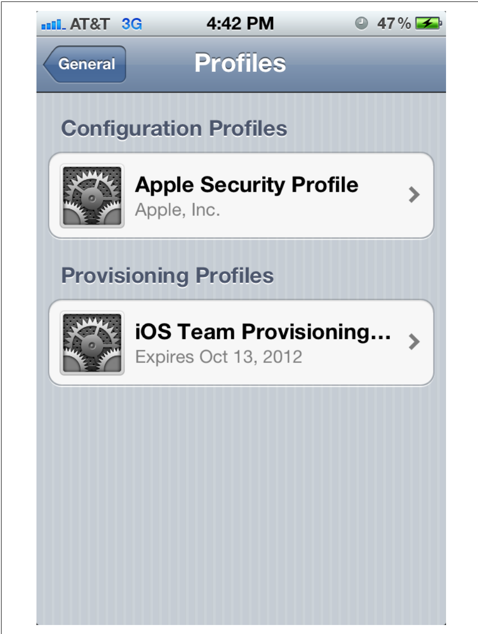
Figure 9-4. Forged configuration profiles do not alert the user to the fact that they are unsigned until clicked on.
